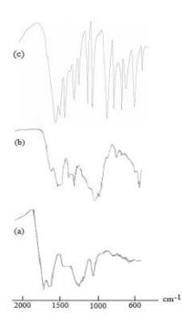
Figure 3: FTIR spectra of HA (a) Aminotriazole-AH complex (b) Aminotriazole (c)
