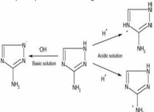
Figure 1: Proposed mechanism of Amatole ions formation in acidic and basic media.
